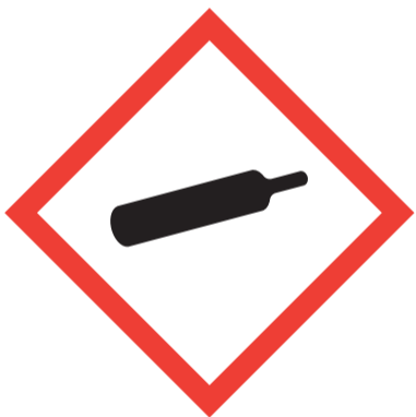
Gas under pressure
